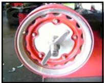
**Balance 'em right.** I am making these adapters for spin balancing 1936 -39 Ford wheels and tires. They are manufactured on a CNC water cutting machine --Royce Hulsey [Royce36@aol.com](mailto:Royce36@aol.com)
