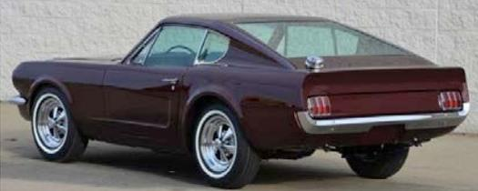
**'Stolen' shorty Mustang.** Ford built this experimental two-seat fastback Mustang from a pre-production chassis shortened 16 inches and stuffed with a 260-cu.in. V-8 bored and stroked to 302 cubic inches. Designer Vince Gardner came up with the fastback profile to fit the shortened wheelbase, which Dearborn Steel Tubing – the same company responsible for the Ford Thunderbolt – rendered in fiberglass with a prominent
